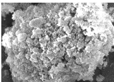
Naomi's Nucleants are made from bio-glass material ( $\text{CaO-P}_2\text{O}_5\text{-SiO}_2$ ) and has a highly porous surface with cavities of similar sizes to proteins. It is hypothesised that the cavities entrap protein molecules, thereby encouraging nucleation and crystal formation.
