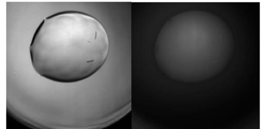
Salt crystals , visible in the brightfield image (above left) are distinguished from protein by the lack of a fluorescence image (above right).
